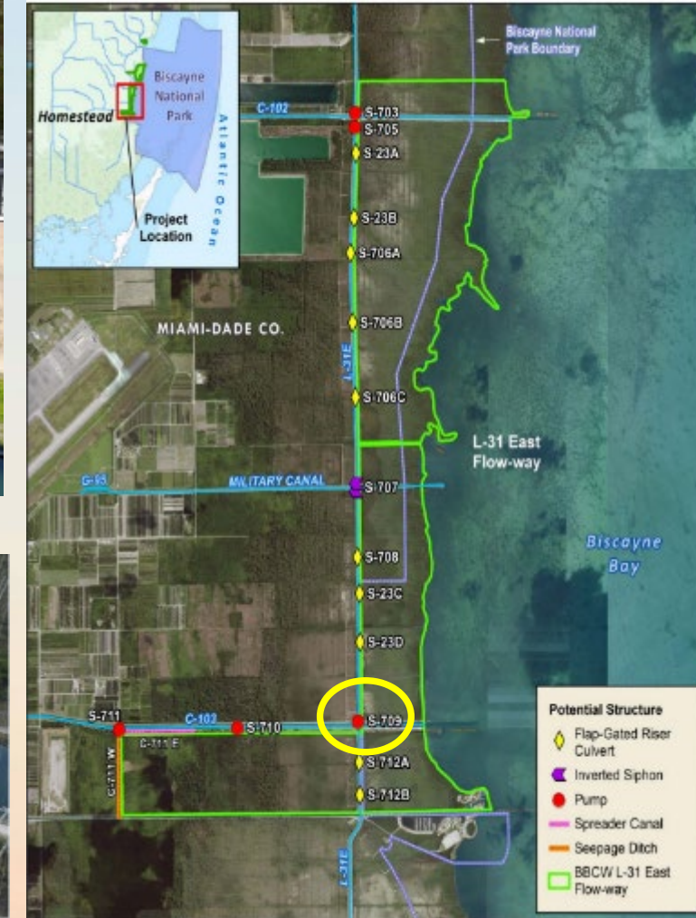
L-31E Flow-way component features
